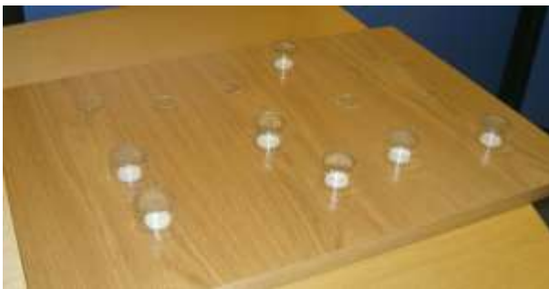
Filter pads with liquid on the surface that is being tested. The pad is covered with a glass cup so the liquid does not evaporate.
